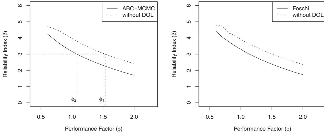
**Figure 8.**  $\phi - \beta$  relationship for ABC-MCMC and Foschi's estimates. When the DOL effect is considered, it can be seen that more failures are expected (and thus a lower reliability index) across all values of  $\phi$  due to damage accumulated from sustained loads. The ABC-MCMC approach provides slightly lower estimates of  $\beta$  overall compared to Foschi's original estimates.
